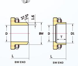
3PC BALL VALVE THRED END&BUTT WELD END
